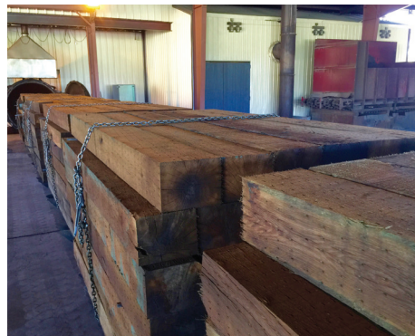
A fresh batch of dual-treated borate-copper naphthenate ties were on the drip pad.
